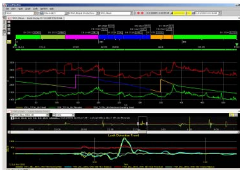
Leak Detection screen in the VisualPipeline GUI.
